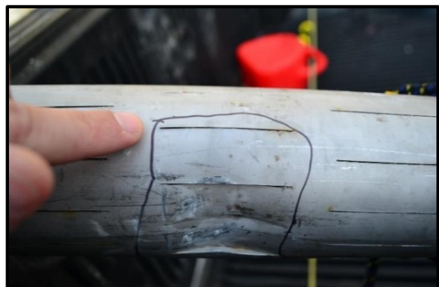
Figure 9. Well Screen Damaged during Horizontal Well Installation at NASNI
