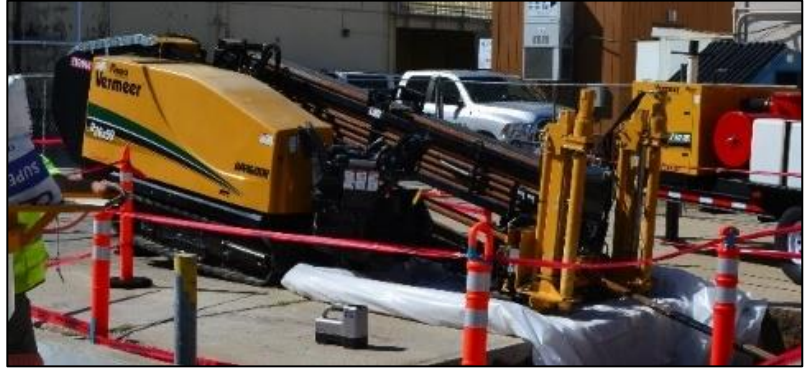
Figure 2. Common Directional Drilling Rig
